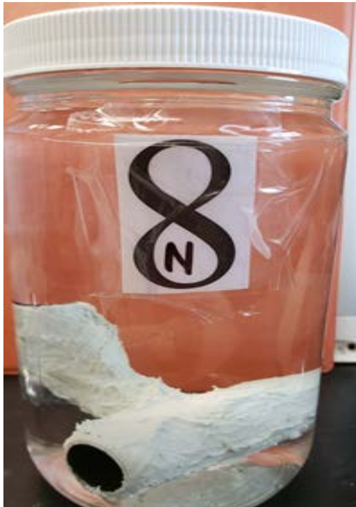
Epoxied Copper Joints with Lead Solder
